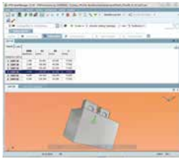
Selection of punch BOLT LOCK, blank according to the max. dimensions of the cutting form Size 04 (A1 x B1 : 120 x 80 mm)
